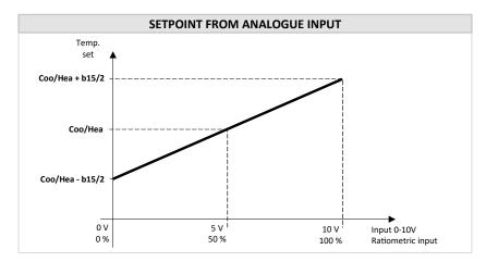
Correction calculation with ratiometric input (b20=1):
